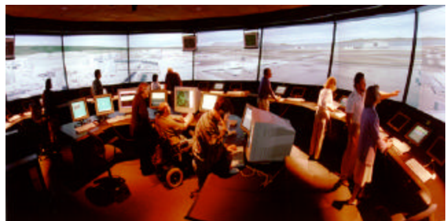
Figure 3. NASA's “FutureFlight Central” is a full-scale virtual airport control tower used to test solutions for potential air and ground traffic problems at commercial airports. The proposed Operations Testbed facility would be similar in function to Flight Central but with a focus on space operations rather than air operations. (image courtesy NASA)
