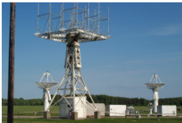
RADAR instrumentation at the Wallops Flight Facility in Virginia tracks suborbital launch vehicles and aircraft.
