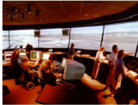
NASA's FutureFlight Central simulates ground operations at major airports around the world. The Intelligent Launch and Range Operations Testbed adapts this concept to space launch operations.
